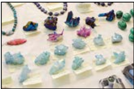
Aqua Aura (pale blue) and Titanium Rainbow Quartz (dark) are just common quartz specimens covered by metal vapor under vacuum. Photo: Zbyněk Buřival
