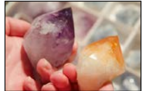
Heat treated amethyst from Brazil gets the typical orange color and is sold as citrine. Photo: Zbyněk Buřival
